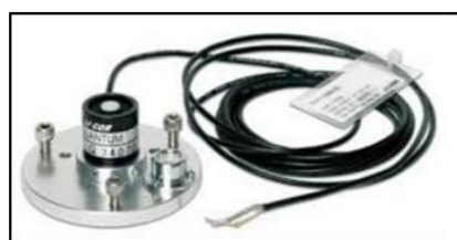
Figure 12. Logger and sensor used to measure the PAR radiation.
