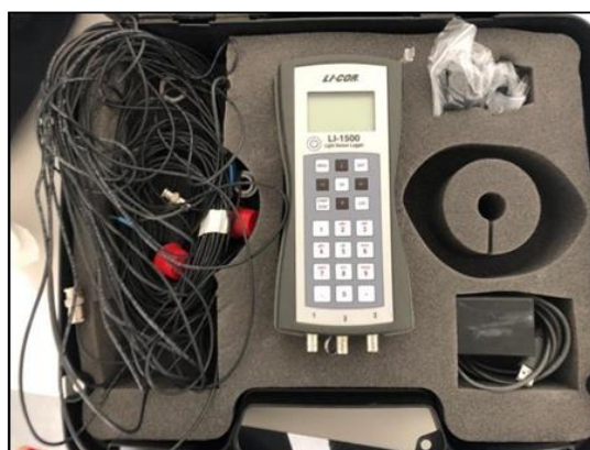
Figure 12. Logger and sensor used to measure the PAR radiation.
